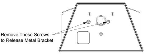
2. In the next step, the metal bracket is attached to the back of the touch screen. To proceed, place the touch screen, face down, on a clean, soft surface.
