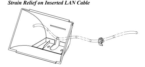
4. Attach the strain relief to the TSW-550/750/1050-TTK by pushing it upward into the slot on the rear of the TSW-550/750/1050-TTK, as shown in the following illustrations.
