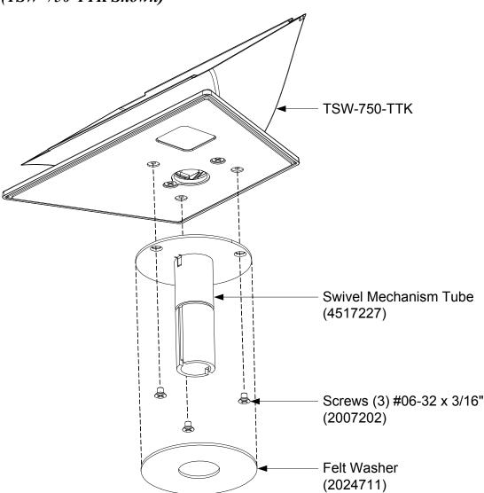
Attaching Swivel Mechanism Tube to TSW-550/750/1050-TTK (TSW-750-TTK Shown)
