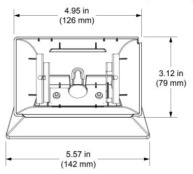
TSW-550-TTK Overall Dimensions (Side View, Shown Without and With TSW-550 Installed)
