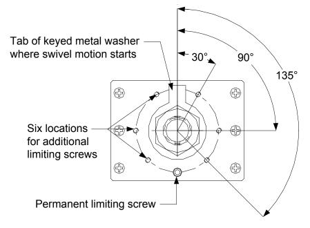
Swivel Stop Plate with Additional Limiting Screws
