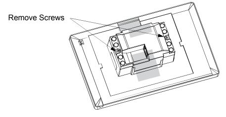
4. Place the metal bracket from step 1, in position on the rear assembly of the touch screen, ensuring it is correctly oriented (right side up) and attach it using the two #04-20 x 5/8" screws (2007139) included with the TSW-550/750/1050-TTK. To prevent damage to threads, back off each screw until it engages the thread. Then tighten to 3 in/lb. Refer to the following illustration.
