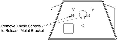
2. With the metal bracket removed, pull downward on the plastic cover to remove it from the TSW-550/750/1050-TTK.
