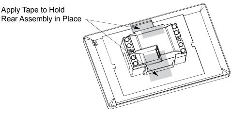
3. Remove the two 1/2" long screws from the rear assembly. Refer to the following illustration. Save these two screws for use if a return to the original configuration is desired.
